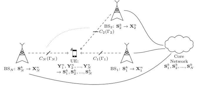
Fig. 1: System model with a single UE,  $N$  base stations, and a core network for the downlink.
