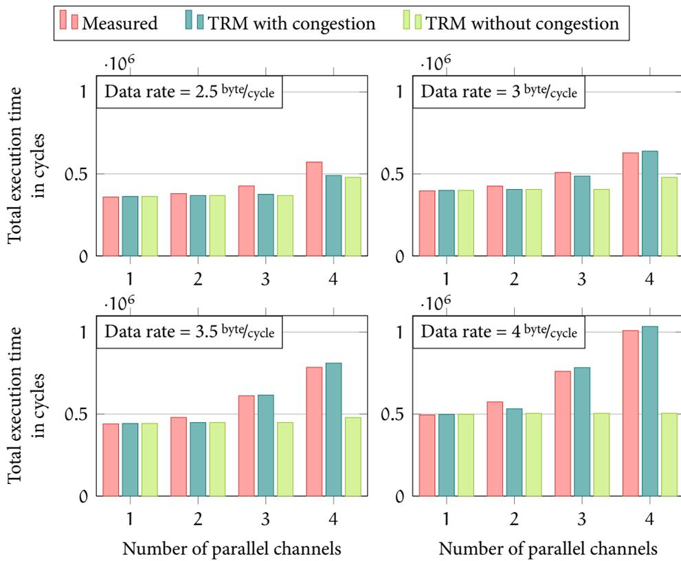
FIGURE 5.8: Comparison of measured execution times and predictions for congestion on a PE link. For high congestion, the congestion model yields accurate predictions.
