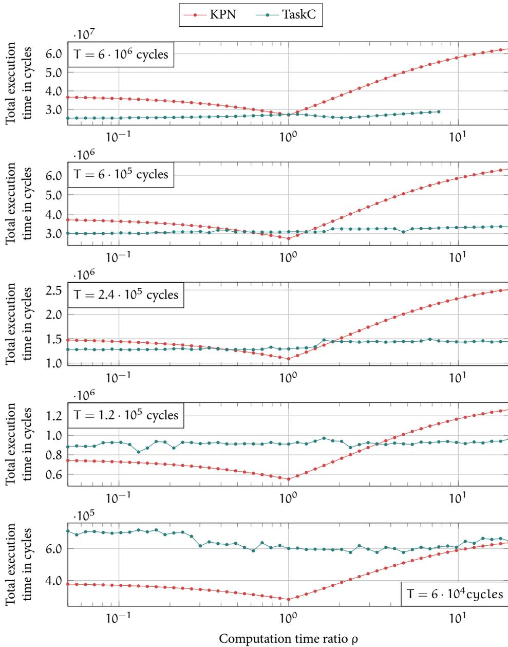
FIGURE 5.12: Performance comparison for the audio filter implemented in TaskC and KPN. The performance of the KPN implementation highly depends on  $\rho$ , which is the ratio between the computation length of filter and FFT.
