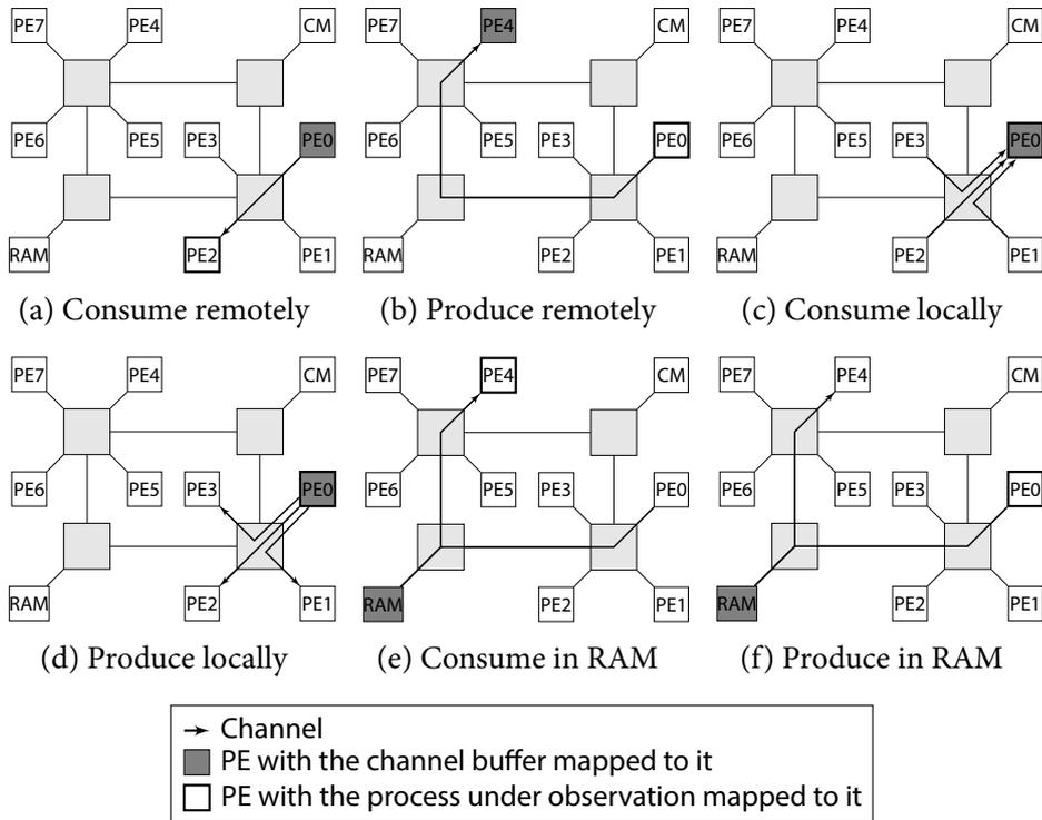
FIGURE 4.1: These experimental setups are used for measurement of communication costs. Each setup applies a different mapping.
