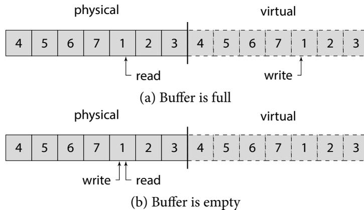
FIGURE 3.2: The channel library uses buffer mirroring for full/empty detection.
