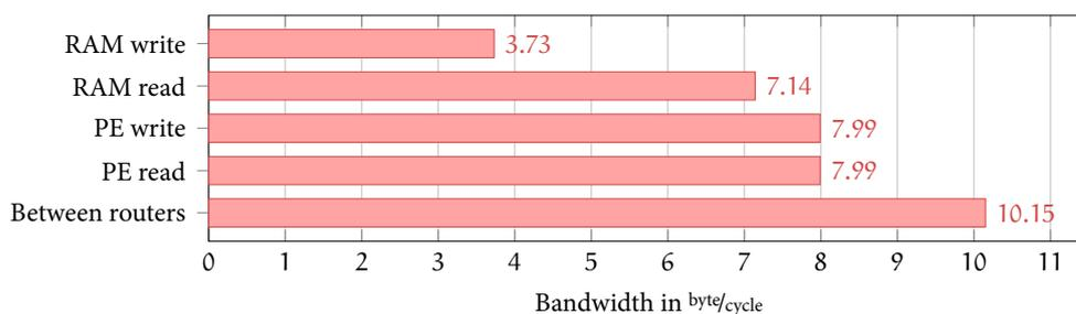
FIGURE 4.5: The measured bandwidths for all five types of links on the Tomahawk2
