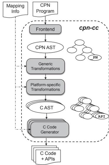
FIGURE 2.4: The code generator creates C code for all target cores. It implements a CPN aware frontend that creates a CPN AST and transforms this AST in order to derive a plain C AST. (Reprinted from [47], © 2013 ACM)
