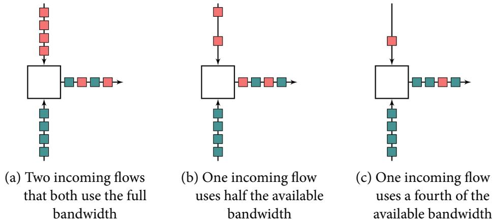
FIGURE 4.7: Contention between two flows can lead to congestion. The slowdown is larger for flows with high data rate and smaller or for flows with low data rate.
