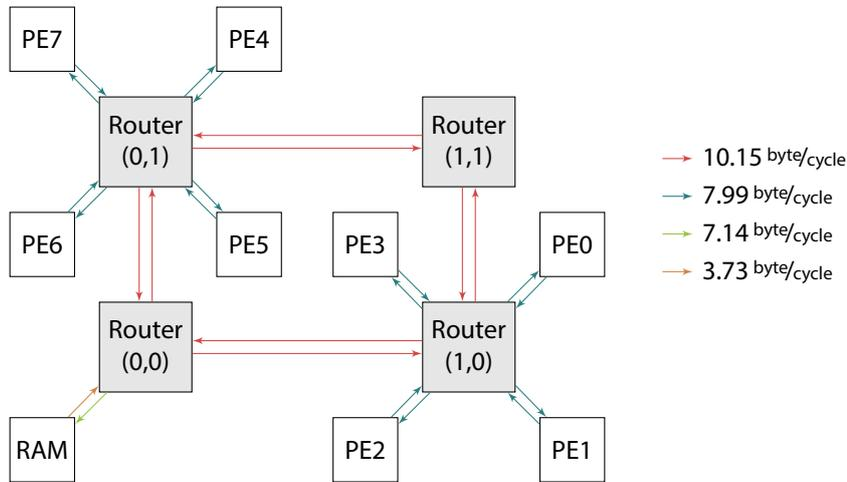
FIGURE 4.6: NoC model for the Tomahawk2 with defined link bandwidths
