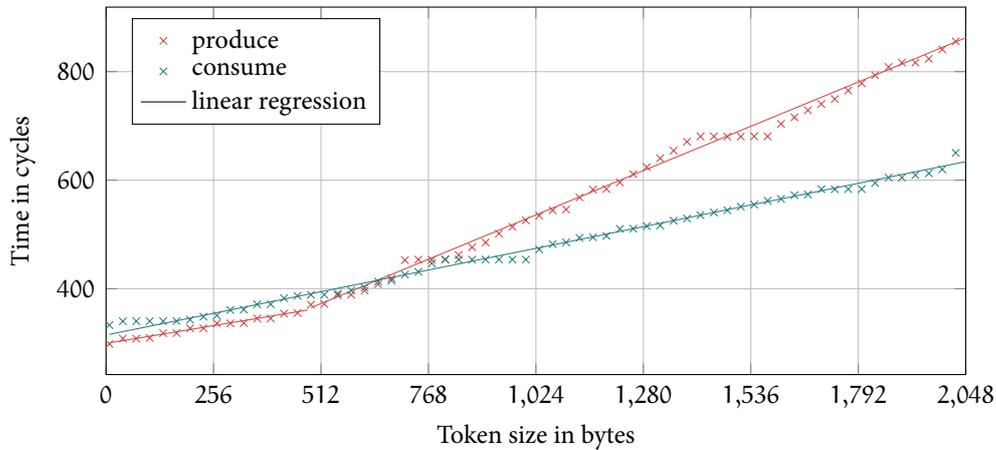
FIGURE 4.3: The measured communication costs for RAM channel accesses do not have a clear linear trend. Nevertheless, the costs are modeled with linear functions.
