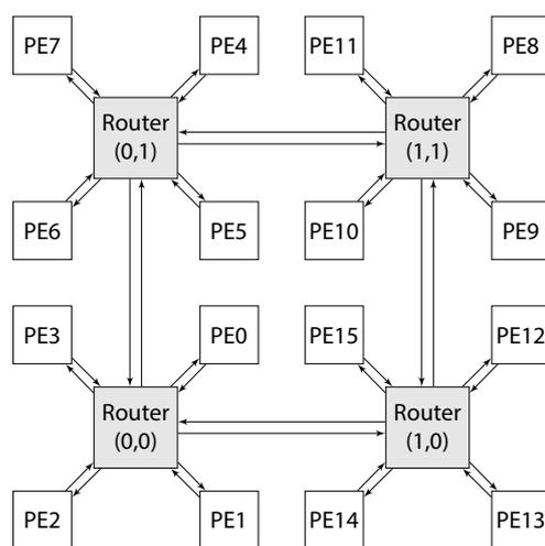
FIGURE 5.14: A virtual platform that represents a possible future generation of the Tomahawk chip.
