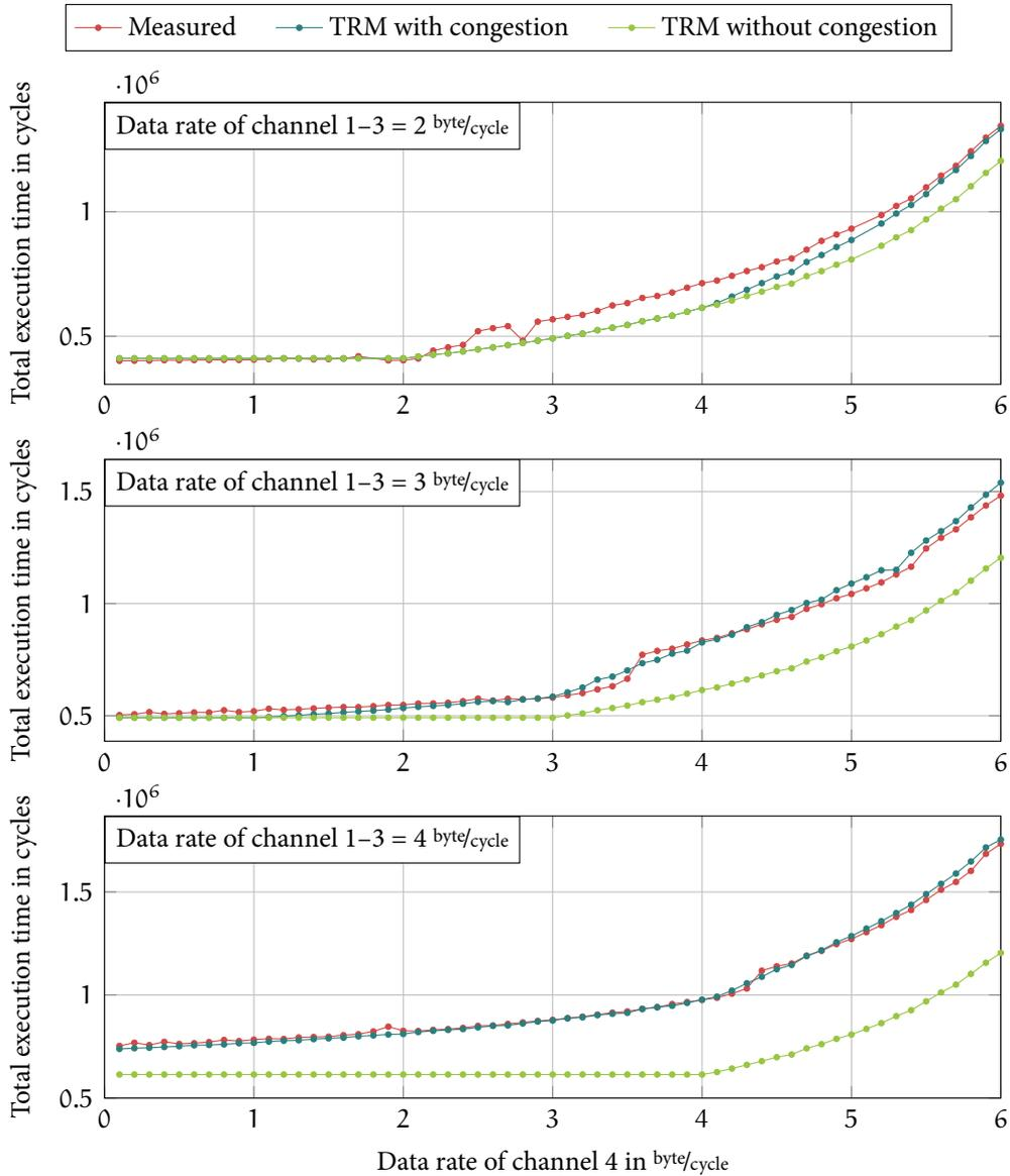
FIGURE 5.9: Comparison of measured execution times and predictions for congestion on a router link. For high congestion, the congestion model yields accurate predictions.
