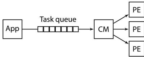
FIGURE 2.5: In the Tomahawk family, the Application Processor (App) issues tasks and the Core Manager (CM) schedules and maps task at runtime.
