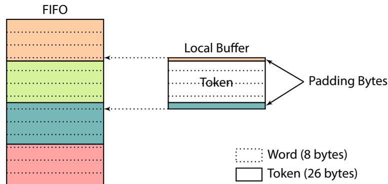
FIGURE 3.4: Due to the eight byte granularity of the Tomahawk2 NoC, writing tokens that have a size that is not a multiple of eight bytes requires padding bytes. The library writes a larger frame and has to fill in the correct padding bytes in order to avoid overwriting valid data.
