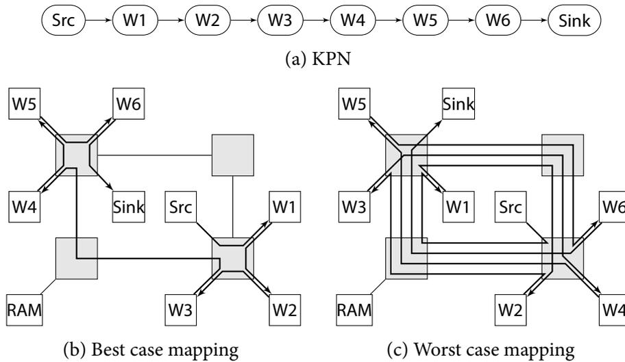
FIGURE 5.3: A pipeline application with two mapping scenarios
