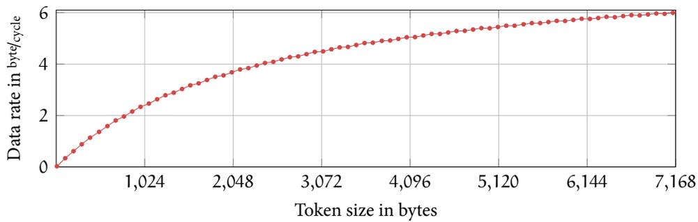
FIGURE 5.7: Relation between token size and average data rate for a single KPN channel
