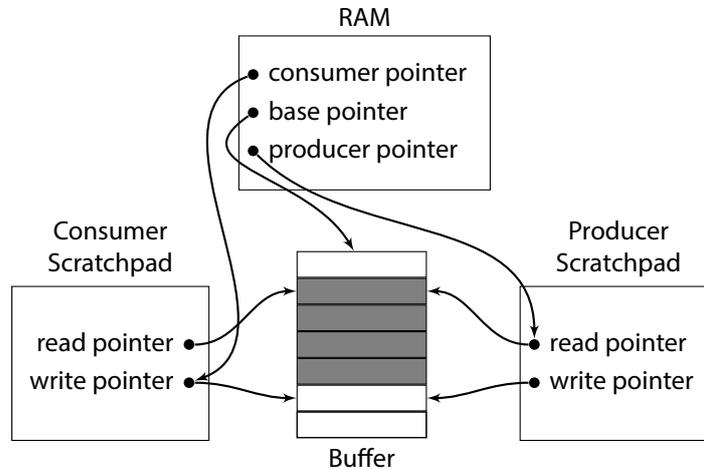
FIGURE 3.3: During initialization, both producer and consumer setup pointers at a known location in global RAM. During execution, these pointers are used to retrieve the position of the circular buffer and to update read or write pointer of the communication partner.
