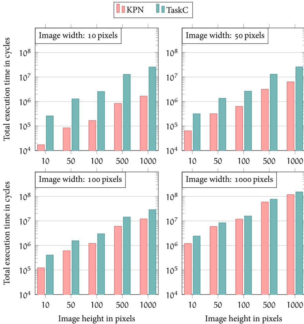
FIGURE 5.11: Performance comparison for the Sobel filter implemented in TaskC and KPN. Although the TaskC application can utilize more PEs, the KPN implementation is always faster.
