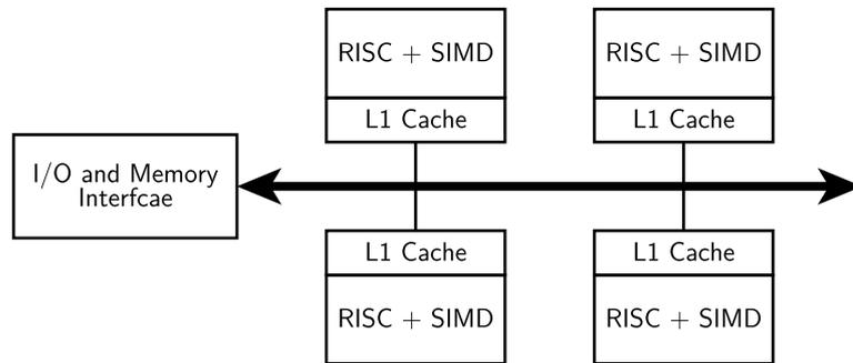
FIGURE 2.1: The Lucent Daytona is the first known MPSoC architecture [1].
