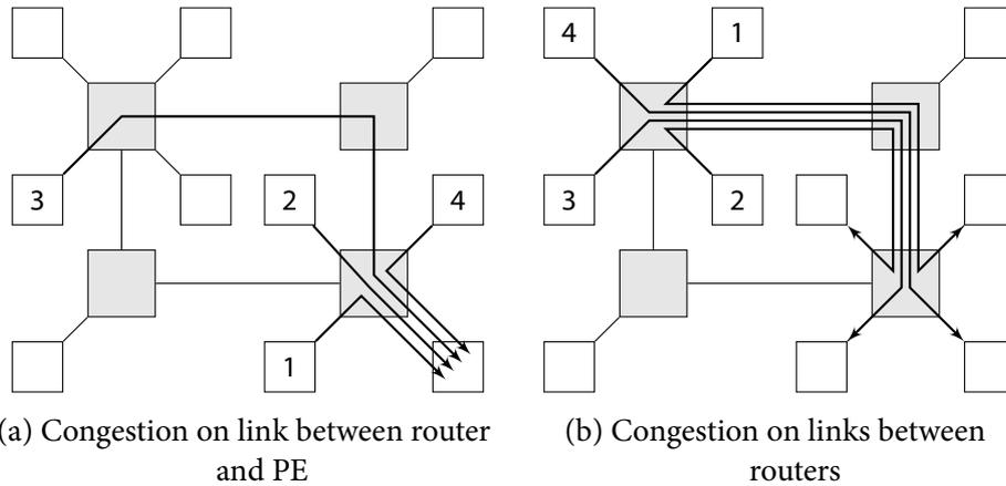
FIGURE 5.6: For the congestion measurement, four parallel channels (labeled 1–4) share certain network links.
