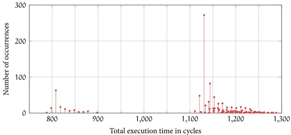
FIGURE 5.1: Distribution of the systematic error over 1,000 time measurements. The median error is 1,141 cycles.
