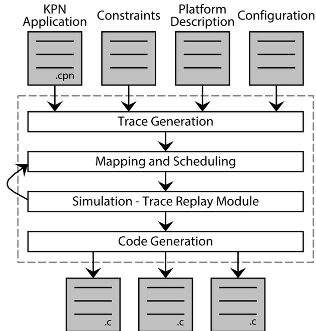
FIGURE 2.2: The MAPS compiler framework provides a complete tool flow for programming MPSoC platforms. It automatically analyzes KPN applications written in CPN, maps them to the target architecture, and generates C code for each target core.
