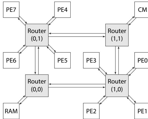
FIGURE 3.1: This simplified model of the Tomahawk2 is used throughout this work. It excludes various features of the Tomahawk2 that are not required for execution of KPN applications.
