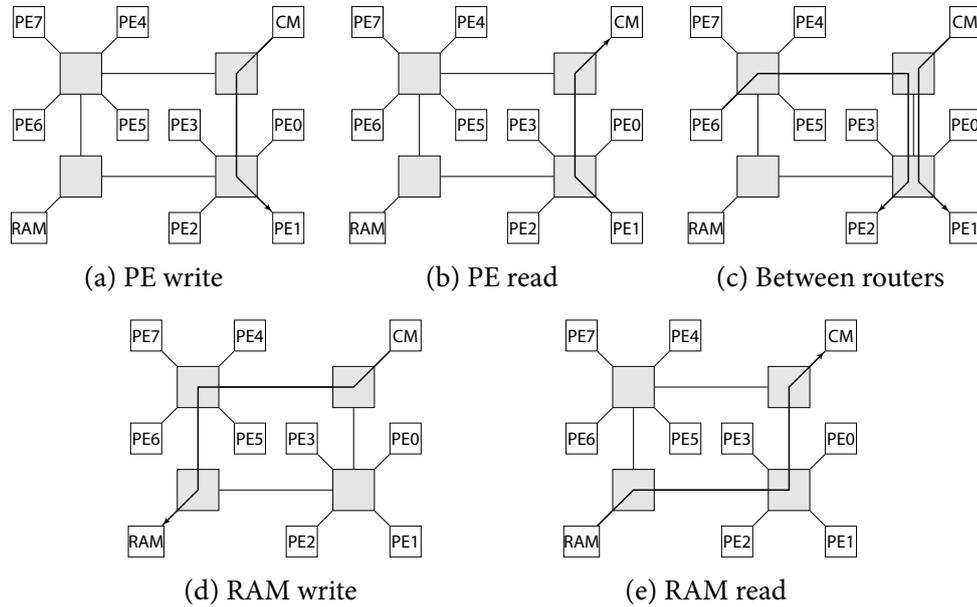
FIGURE 4.4: The experimental setups for measuring the link bandwidth of all five types of links on the Tomahawk2
