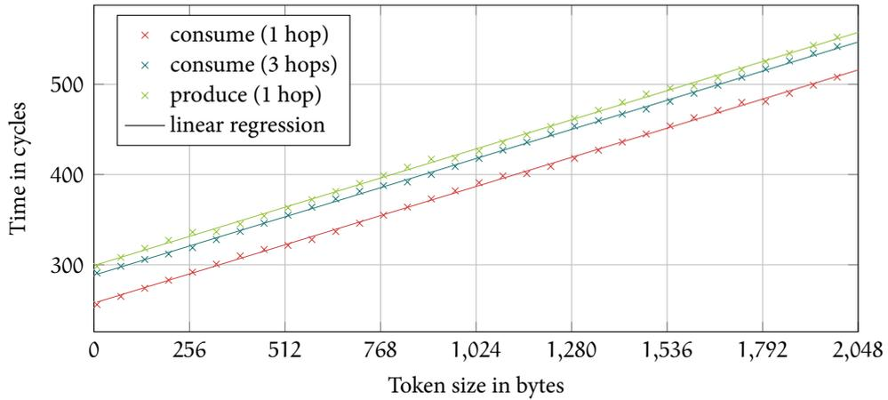
FIGURE 4.2: The measured communication costs for remote channel accesses clearly show a linear trend.
