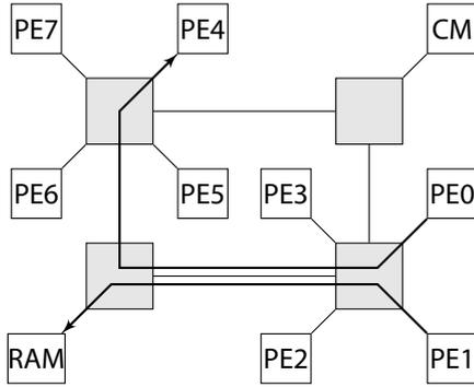
FIGURE 4.8: A flow going to the RAM can fill up the input buffer in the south-west router and thereby block other flows that use the same input port.
