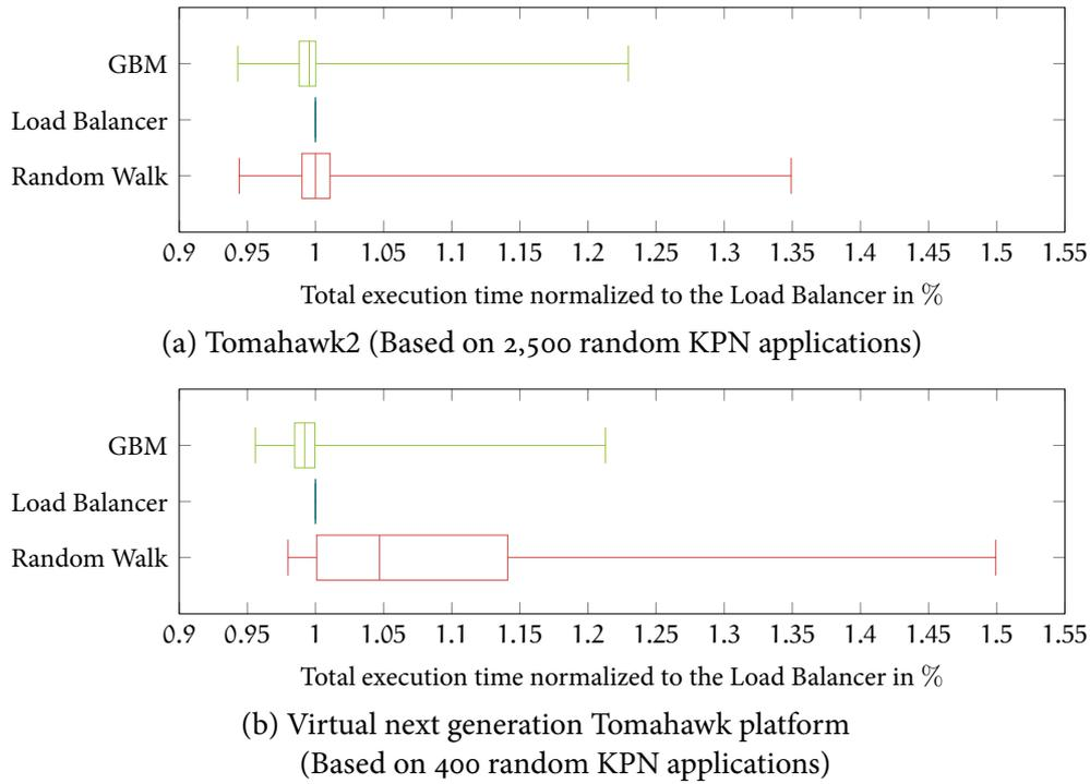
FIGURE 5.13: Box plots comparing the total execution time of three mapping algorithms normalized to the Load Balancer. The more complex GBM algorithm is not significantly better compared to the Load Balancer.
