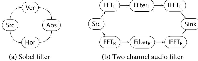
FIGURE 5.10: KPN representation of two applications that are used for performance comparison of KPN and TaskC
