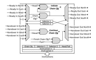
Fig. 8. The synchronizer inside each SubCtrl. It is used to synchronize the connection (de)-activating processes.
