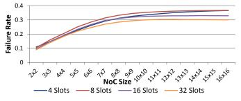
Fig. 14. The failure rate in allocating paths with feedback when the number of time slots is varied. The network utilization is 0.5.
