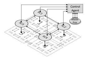
Fig. 7. Example of *distributed control plane* in a 4x4 NoC with 4 *Sub-Controllers* and 1 Control Agent. Each Sub-Controller controls 4 SWs. The Master Proc sends instructions to the Sub-Controllers via the Control Agent.
