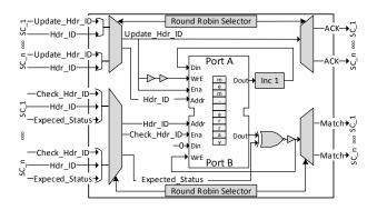
Fig. 9. The synchronizer at the Control Agent to support out-of-order connection activation.
