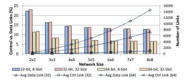
Fig. 12. The ratio between the number of control and data links in various network sizes, data widths and numbers of time slots. The average number of data links and control links are also reported.
