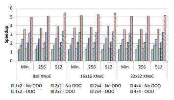
Fig. 16. The speedups gained from distributed control plane in different network sizes, instruction buffer sizes and number of SubCtrls. *The instructions are written directly to SubCtrls by Master Proc.*
