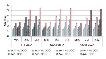
Fig. 15. The speedups gained from distributed control plane in different network sizes, instruction buffer sizes and number of SubCtrls. *The instructions are distributed to SubCtrls by Control Agent*.
