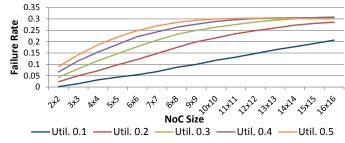
Fig. 13. The failure rate in allocating paths with feedback with varying network utilization. The number of time slots is 32.
