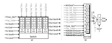
Fig. 4. (a) The 5-input XSwitch. It consists of a set of 5-input memory elements (MEs). The gray signals are from the Control Unit. The ones with asterisk are global. (b) Example of how a multiplexer is realized by changing the content of the ME. The ME is simplified to 3-input for illustration.
