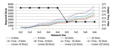
Fig. 11. The synthesis results of XNoC with different configurations.
