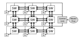
Fig. 3. The 3x3 XNoC. The SWs and NIs are in Data Plane. The PEs (not shown for simplicity) are attached to the NIs. The Control Unit receives instructions from the Master Processor (Master Proc) to control the Data Plane.
