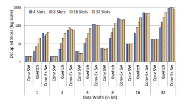
Fig. 10. The resource costs of three SWs with varied numbers of time slots and data widths. The number of slices is obtained after the Mapping phase.
