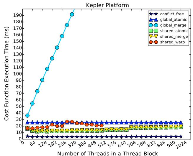
Fig. 10. Execution time for different threads per block in Kepler GPU. *shared\_warp* breaks halfway is due to the shortage of shared memory.
