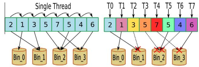
Fig. 2. Update conflicts for histogram calculation on multithreaded platform: If T0 and T2 update Bin 1 simultaneously, one may overwrite the other, leading to incorrect results.
