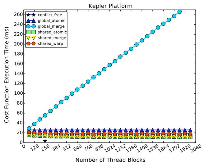
Fig. 7. Execution time for different thread blocks in Kepler GPU.
