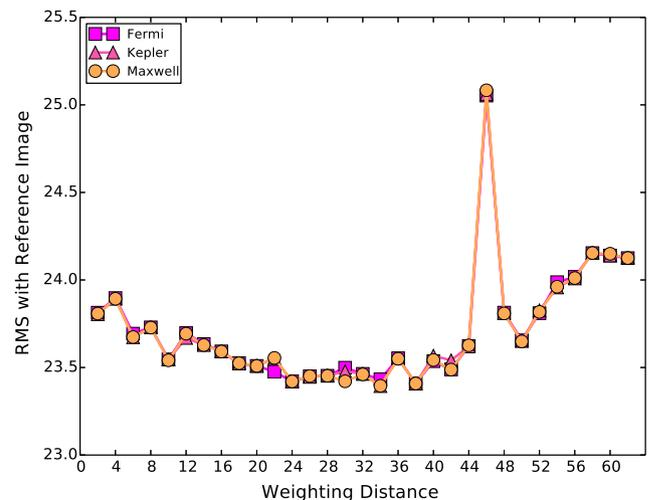
**Fig. 19.** RMS error with the reference image over weighting distance. The curve decreases at the beginning showing that weighting the border region does help to improve global accuracy but if the weighting distance is too large, significant bias are suffered.
