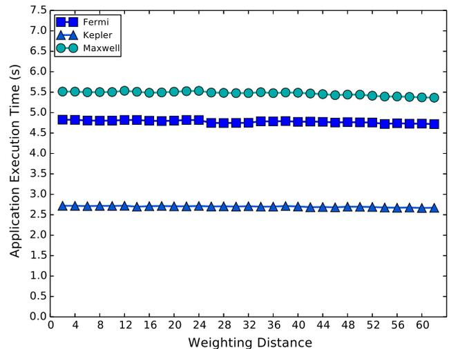
**Fig. 18.** Average execution time over weighting distance. The execution time seems irrelevant to the size of weighting distance indicating that these extra computation overhead are completely hidden by multithreading and the long latency texture fetching.
