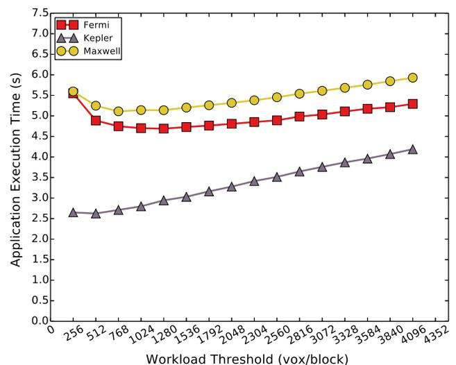
**Fig. 17.** Average execution time over the maximum per-block workload. The curve drops drastically at the beginning and increases thereafter indicating that after the flex point, the impact of load unbalancing appears to be prominent.
