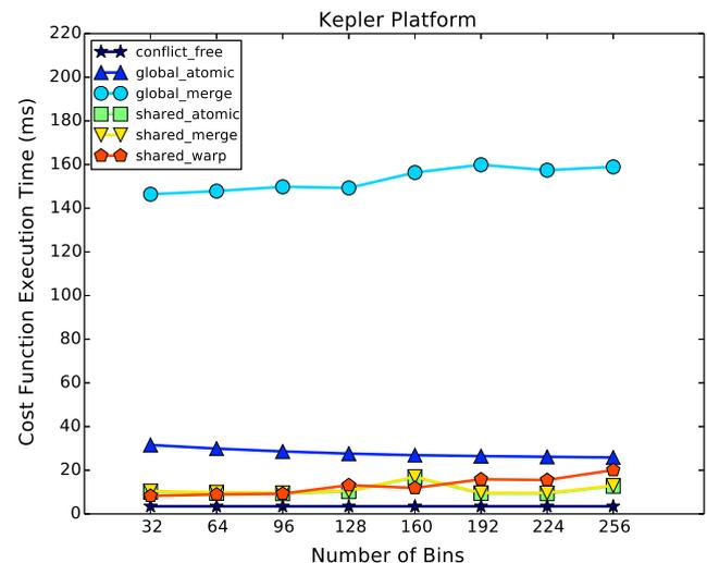
**Fig. 13.** Execution time for different histogram bins in Kepler GPU.
