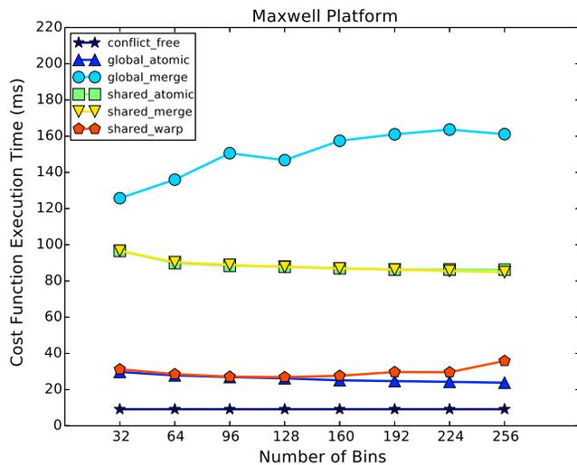
Fig. 14. Execution time for different histogram bins in Maxwell GPU.
