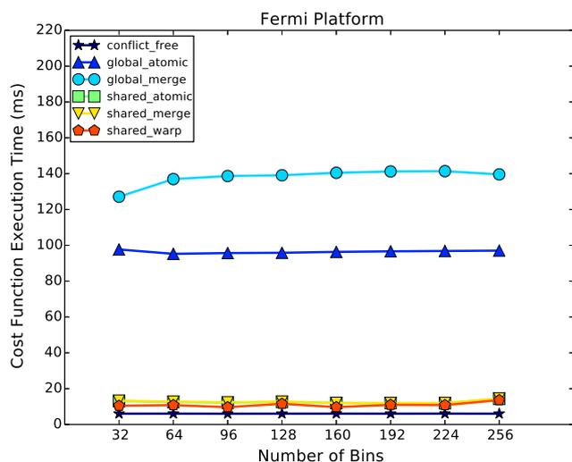
**Fig. 12.** Execution time for different histogram bins in Fermi GPU.
