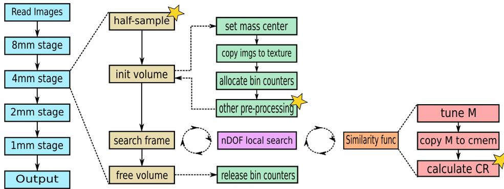
**Fig. 3.** Algorithm framework. The vertical arrows indicate module execution sequences. Dashed horizontal arrows implies module hierarchy. The dashed circle means the right-hand modules are called by the left-hand module repeatedly. The yellow star means the current module contains GPU kernel functions. (For interpretation of the references to colour in this figure legend, the reader is referred to the web version of this article.)
