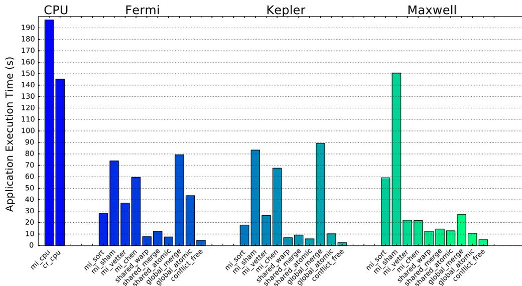
Fig. 15. Application execution time for different schemes on different platforms. As can be seen, *conflict\_free* always shows the best performance, especially on Kepler GPU.
