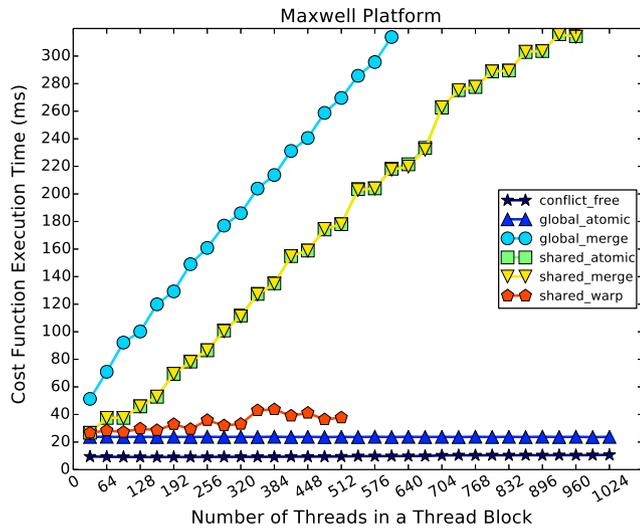
**Fig. 11.** Execution time for different threads per block in Maxwell GPU. *global\_merge* and *shared\_warp* break halfway are due to the shortage of global memory and shared memory.
