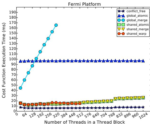
Fig. 9. Execution time for different threads per block in Fermi GPU. *global\_merge* and *shared\_warp* break halfway are due to the shortage of global memory and shared memory.
