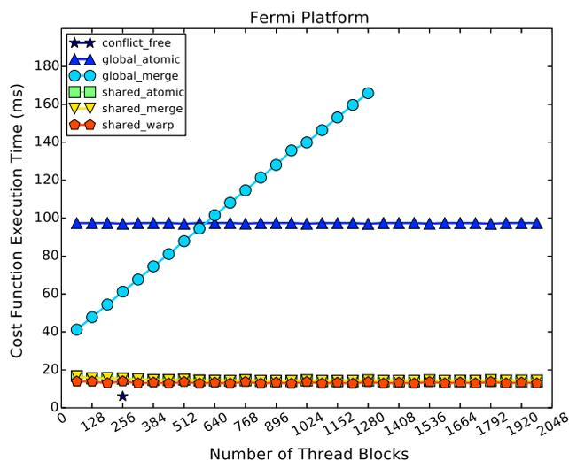
Fig. 6. Execution time for different thread blocks in Fermi GPU. *global\_merge* breaks halfway is due to the shortage of global memory.
