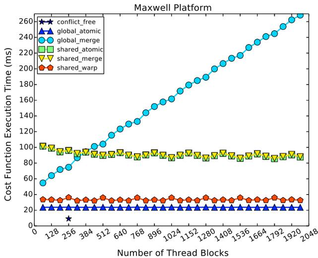
Fig. 8. Execution time for different thread blocks in Maxwell GPU.
