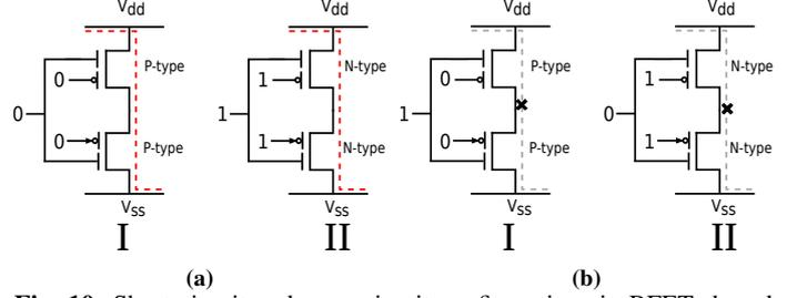
**Fig. 10:** Short-circuit and open-circuit configurations in RFETs-based inverters.
