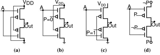
**Fig. 9:** Connections for inverters [60] (a) Static design. The drain, source and program gate are hard fixed to  $V_{dd}$  and  $V_{ss}$  (b) One transistor’s program terminal is connected to 0 (c) One transistor’s program terminal is connected to 1 (d) Fully reconfigurable design.
