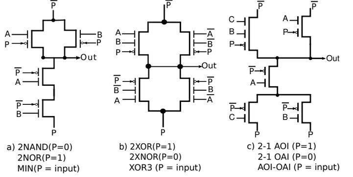
Fig. 7: Reconfigurable logic gates using RFETs [60]
