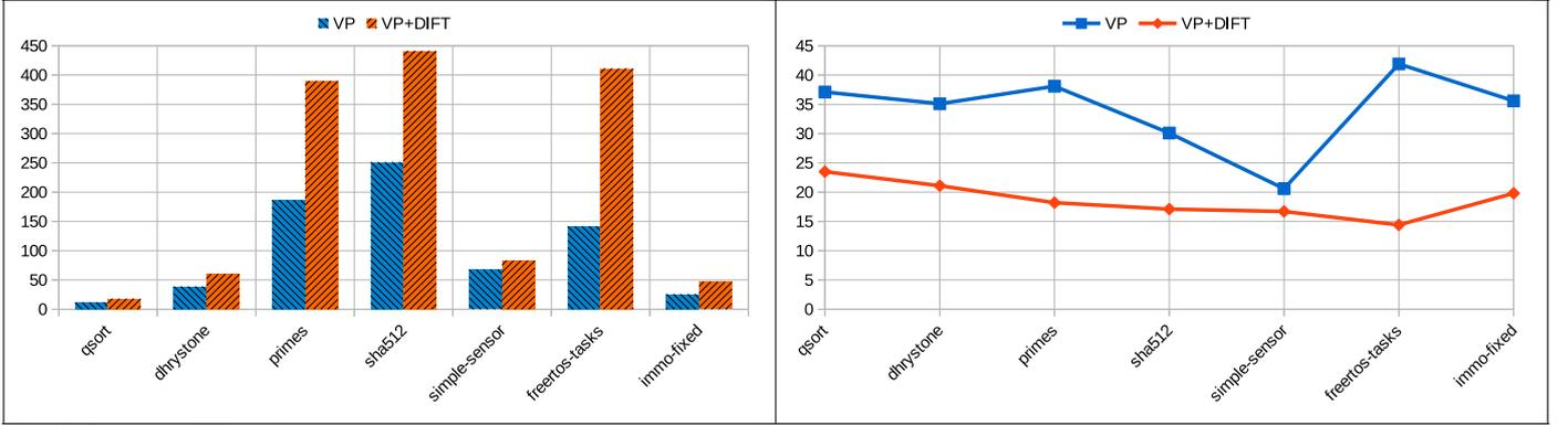
**Fig. 4:** Dynamic IFT performance overhead evaluation results - the left side shows the execution time in seconds and the right side the achieved MIPS for the normal VP (blue color) and the VP with dynamic IFT integration (orange color).
