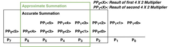
Fig. 3.  $4 \times 4$  multiplier using two  $4 \times 2$  multipliers [14].
