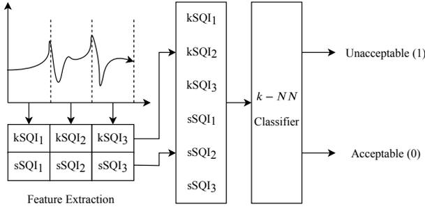
Fig. 1. Flow diagram of the proposed methodology with the details of the SQI features extracted (kSQI and sSQI) discussed in Section III.
