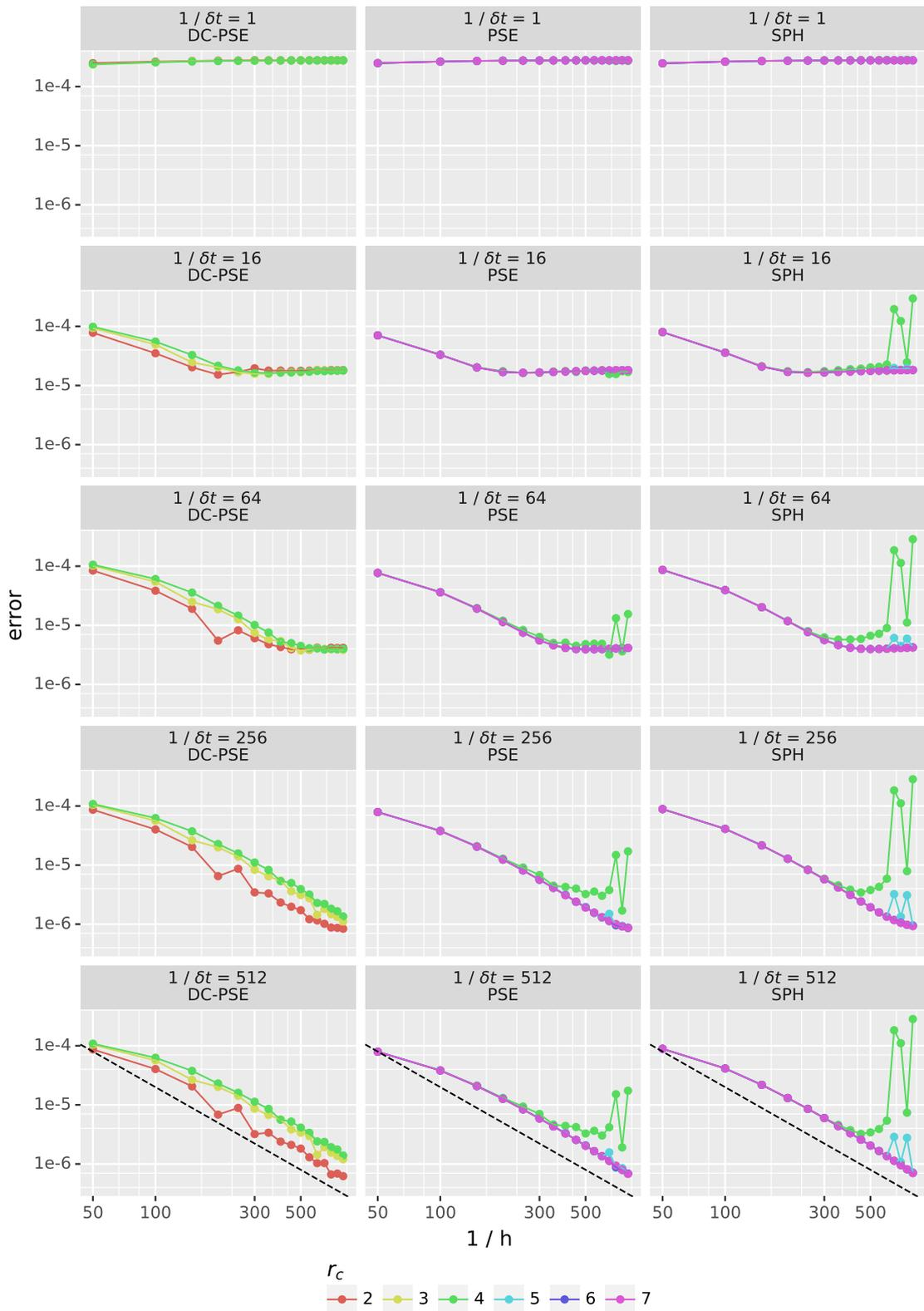
Figure 5.4.: Gray-Scott parameter study relating the error, spatial and temporal resolution and discretization method. The dashed line has a slope of -2 representing quadratic relations in the logarithmic diagram.
