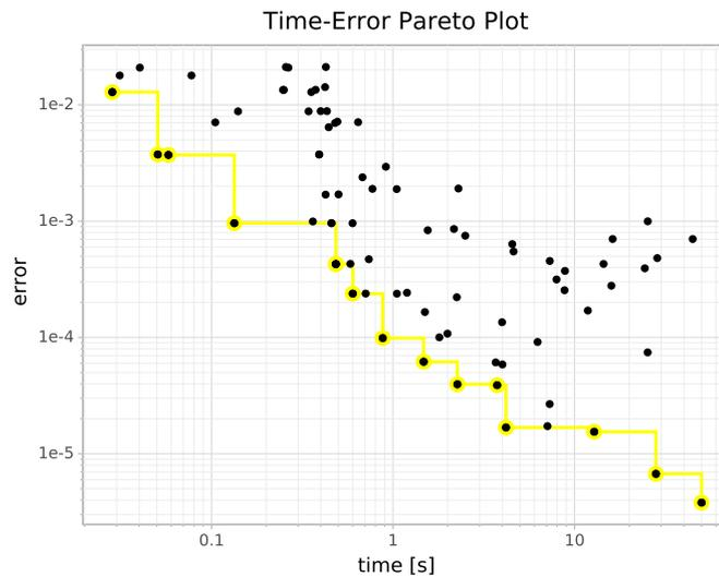
Figure 4.5.: Nondominated configurations in the objectives time and error are connected via the yellow line. Assuming that the whole search space is visualized, those configurations are called Pareto-optimal. Any position above the yellow line is dominated by one of the Pareto elements. The plot uses measurements of the diffusion problem for  $t=0$ , with varying  $\epsilon$ ,  $h$ ,  $r_{cut}$  and discretizations methods.
