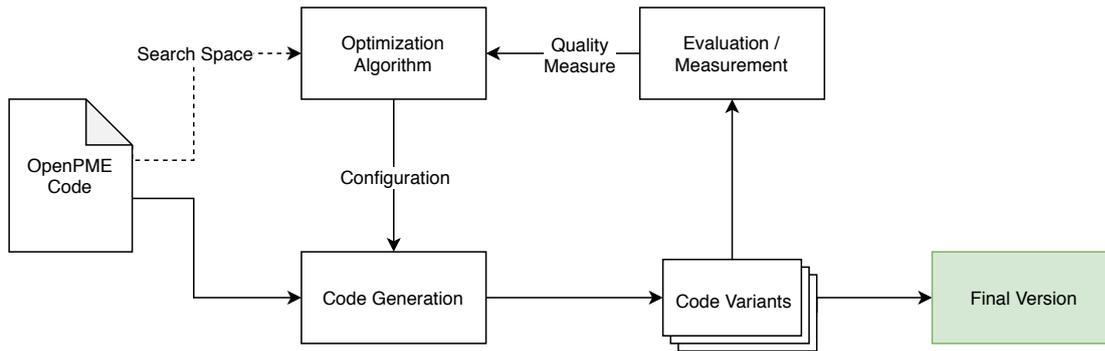
Figure 4.1.: General structure and components of the implemented autotuner.
