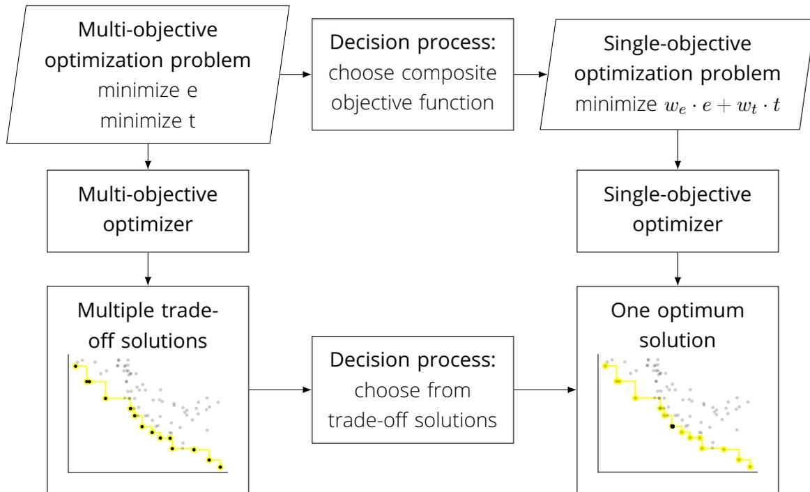
Figure 4.6.: Schematic of the two possibilities for multi-objective optimization procedures based on Deb [21, pp. 408-409].
