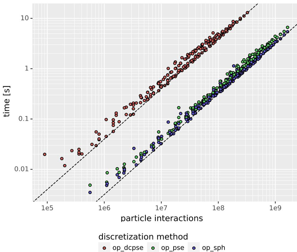
Figure 5.8.: Relation between the number of particle interactions and runtime. The dashed lines have a slope of one and denote linear relationships in the logarithmic diagram.
