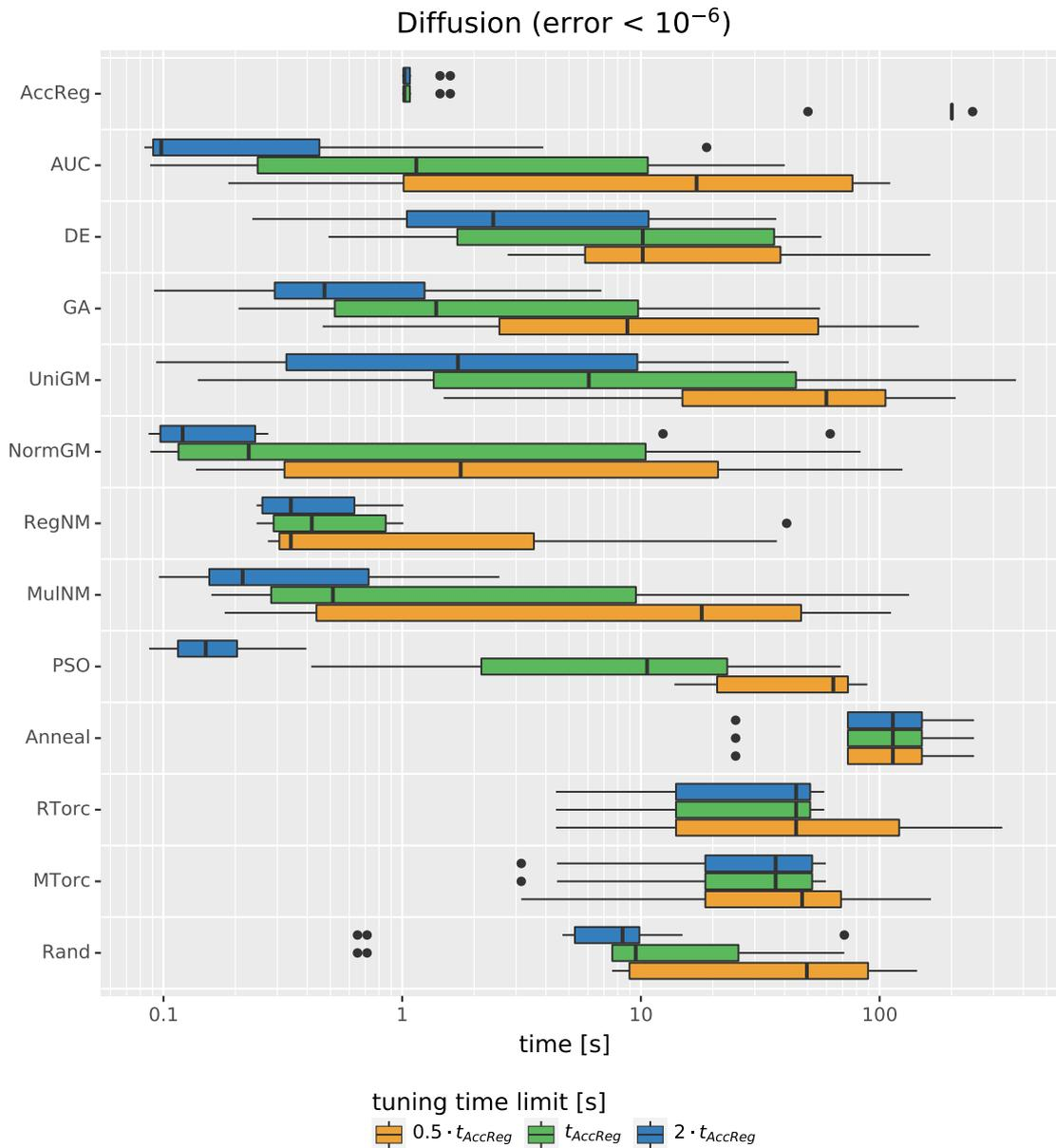
Figure B.2.: Achieved simulation runtimes by different optimization algorithms for the diffusion simulation with an error threshold of  $10^{-6}$ . The runtime (x-axis) refers to the measured time over the tuning period ( $t = 0$  to  $t = 2$ ). Each algorithm is evaluated with an upper tuning time limit of 0.5, 1 and 2 times the tuning time of the model-based search.
