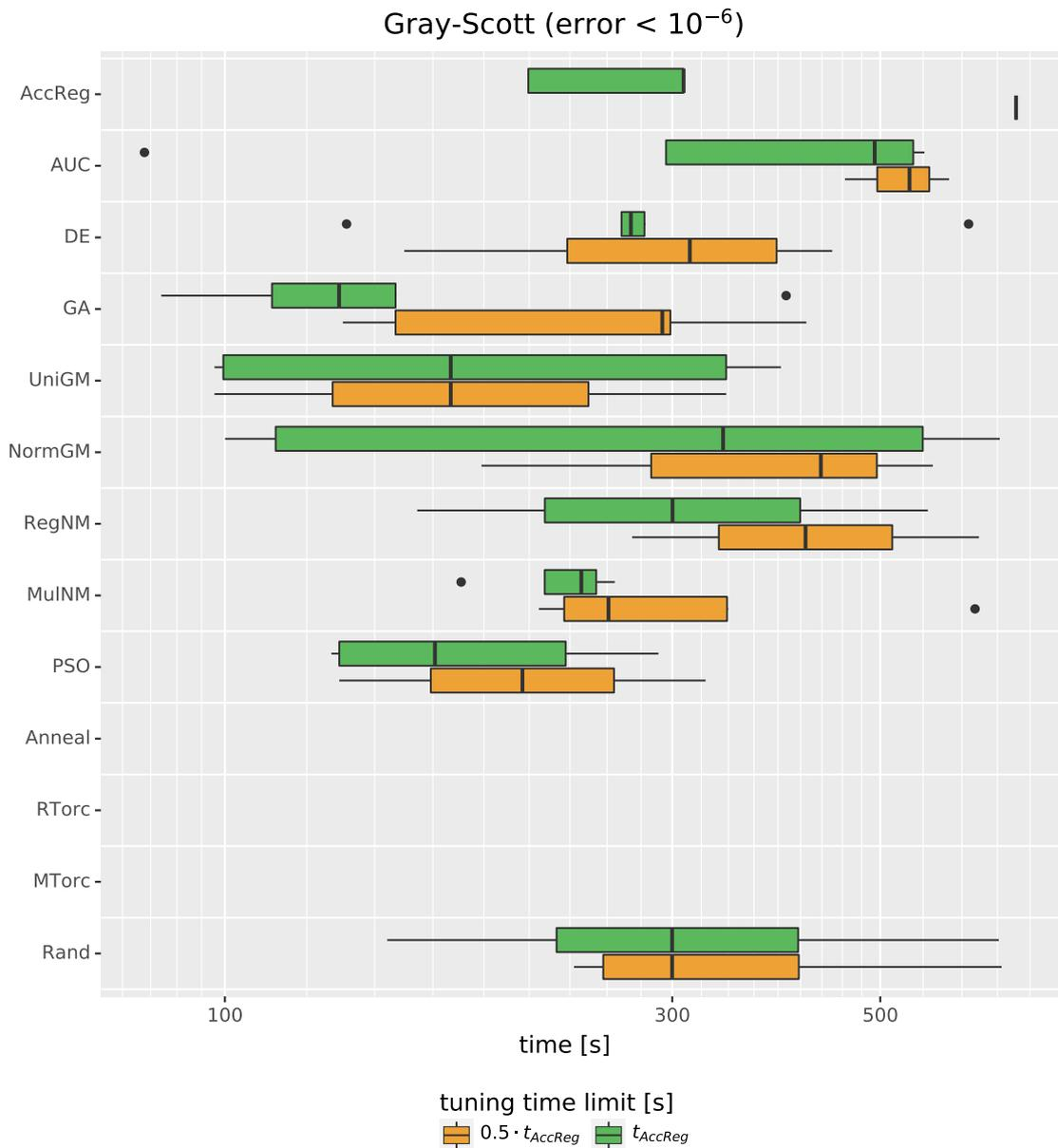
Figure B.4.: Achieved simulation runtimes by different optimization algorithms for the Gray-Scott simulation with an error threshold of  $10^{-6}$ . The runtime (x-axis) refers to the measured time over the tuning period ( $t = 0$  to  $t = 2$ ). Each algorithm is evaluated with an upper tuning time limit of 0.5 and 1 times the tuning time of the model-based search.
