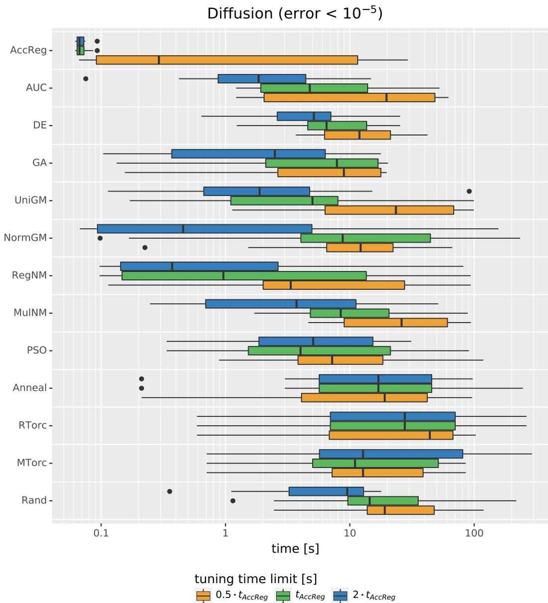
Figure B.1.: Achieved simulation runtimes by different optimization algorithms for the diffusion simulation with an error threshold of  $10^{-5}$ . The runtime (x-axis) refers to the measured time over the tuning period ( $t = 0$  to  $t = 2$ ). Each algorithm is evaluated with an upper tuning time limit of 0.5, 1 and 2 times the tuning time of the model-based search.
