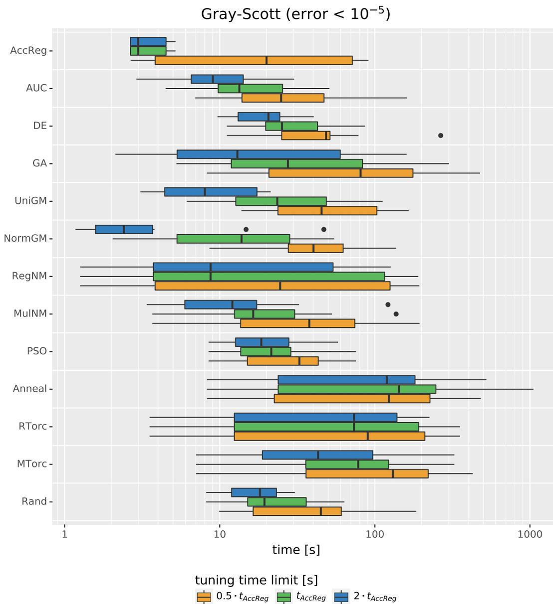
Figure B.3.: Achieved simulation runtimes by different optimization algorithms for the Gray-Scott simulation with an error threshold of  $10^{-5}$ . The runtime (x-axis) refers to the measured time over the tuning period ( $t = 0$  to  $t = 2$ ). Each algorithm is evaluated with an upper tuning time limit of 0.5, 1 and 2 times the tuning time of the model-based search.
