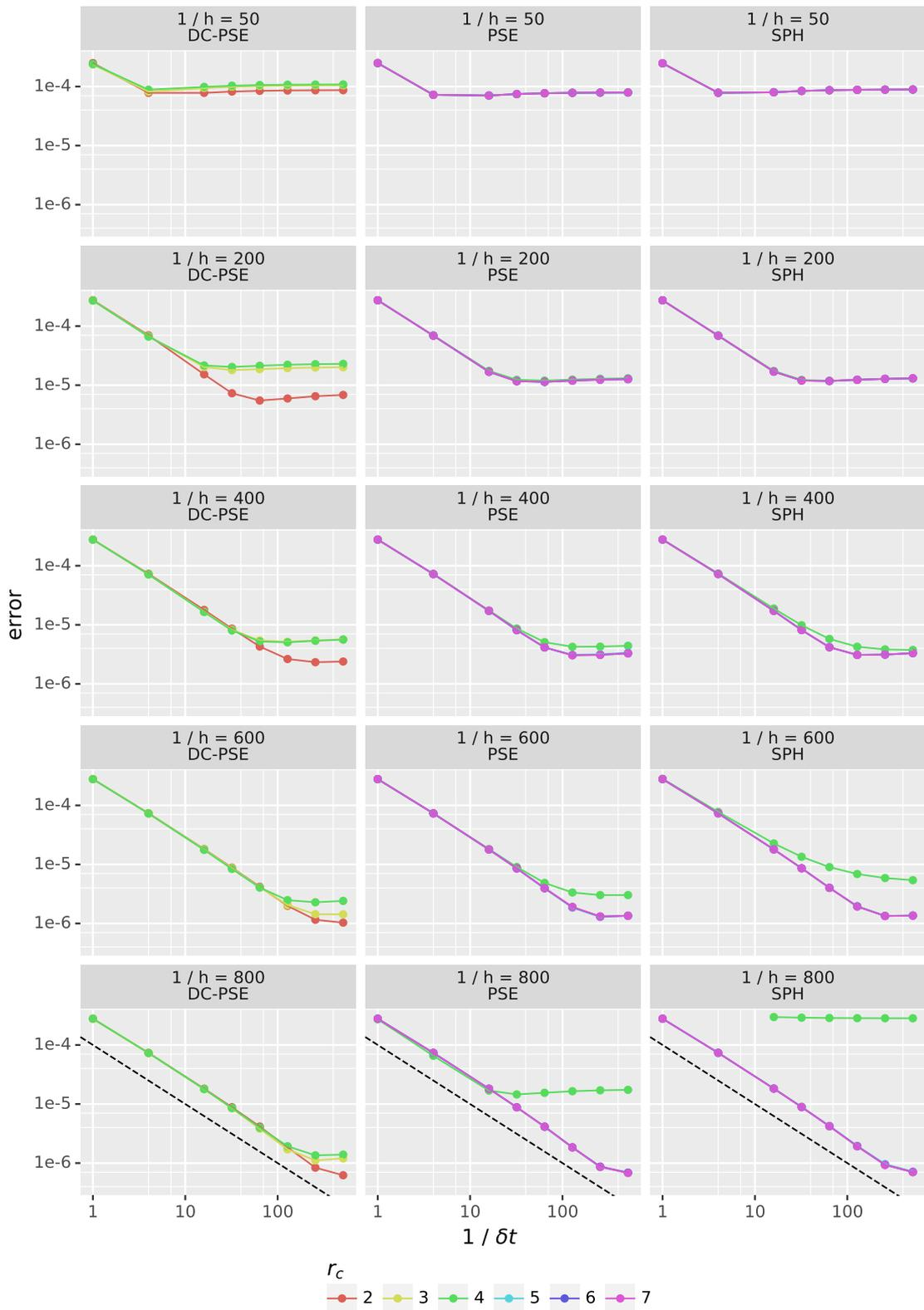
Figure 5.7.: Gray-Scott parameter study relating the error, temporal and spatial resolution and discretization method. The dashed line has a slope of -1 representing linear relations in the logarithmic diagram.
