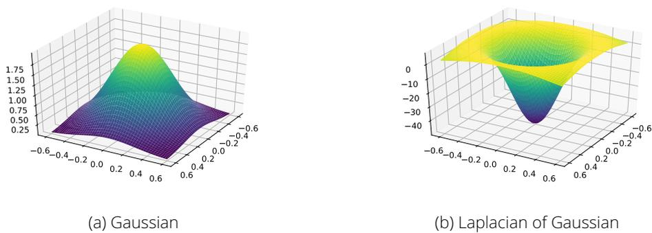
Figure 3.1.: Initial condition used in the diffusion simulation along with its Laplacian.
