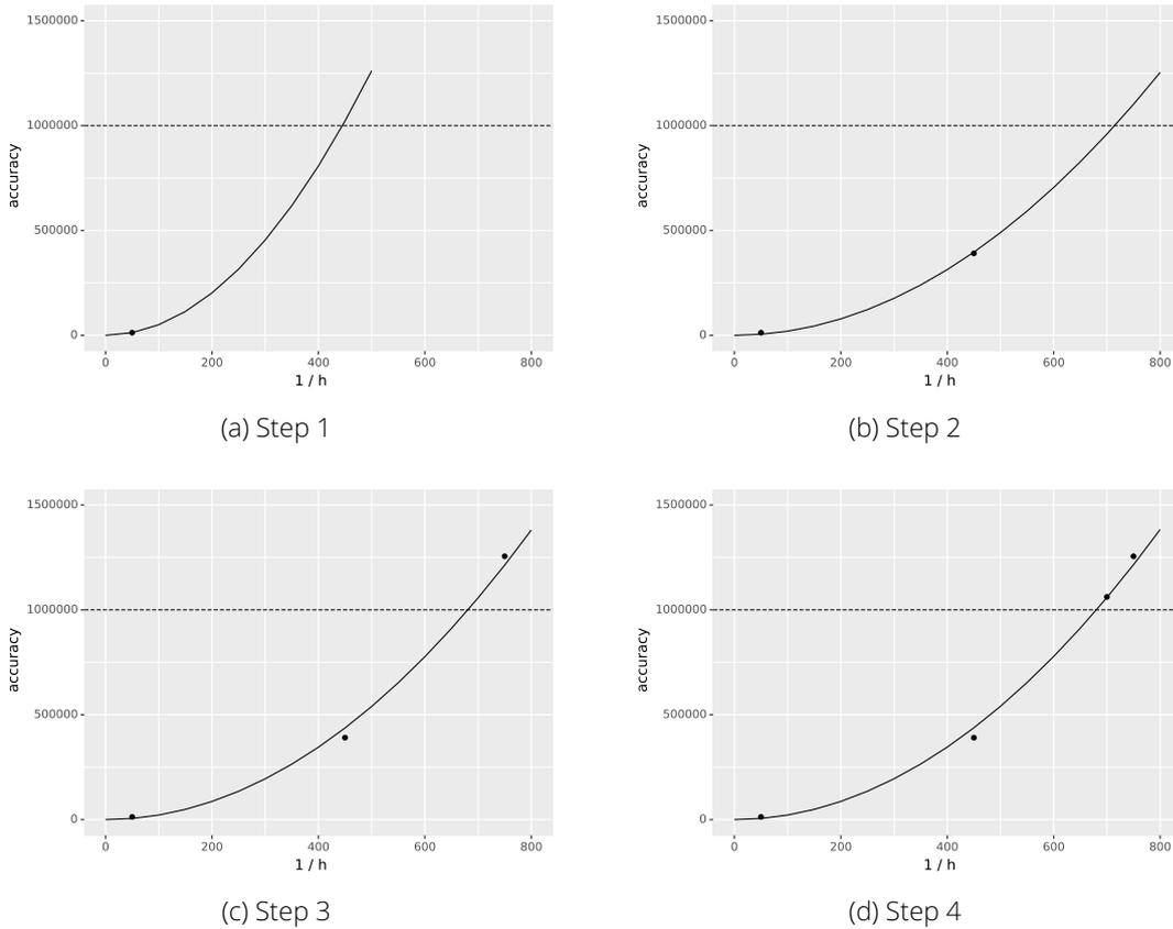
Figure 5.6.: Model-based search steps used to optimize  $h$ . The plots use an accuracy value (one divided by the error) rather the error to better visualize the quadratic dependency between error and resolution.
