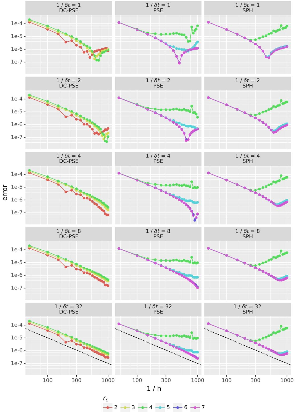
Figure 5.5.: Diffusion parameter study relating the error, spatial and temporal resolution and discretization method. The dashed line has a slope of -2 representing quadratic relations in the logarithmic diagram.
