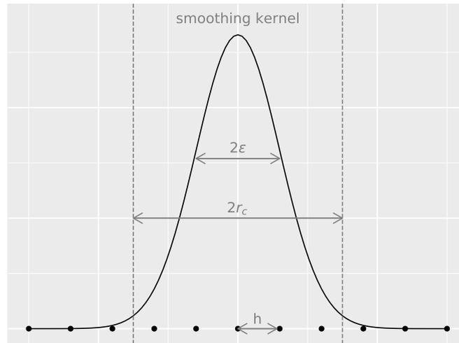
Figure 3.9.: Visualization of tuning parameters. The vertices at the bottom represent particles in 1D with inter-particle distance  $h$ . The function shows a Gaussian smoothing kernel with width  $\epsilon$ . The vertical bars show the neighborhood radius. The influence of the particles beyond is truncated.
