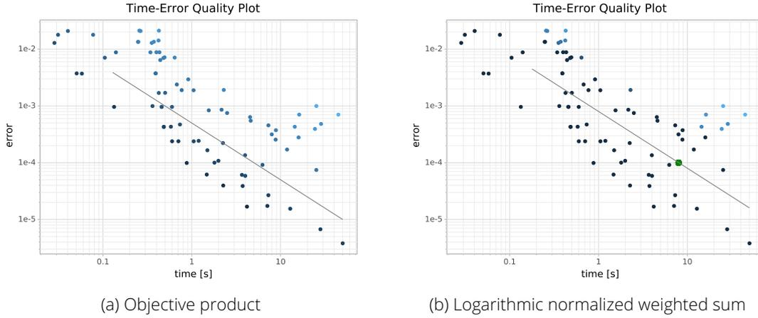
Figure 4.8.: Objective product and the equivalent using weighted sums of logarithms. Points along the line share the same quality while the points below have a higher and the points above a lower quality.
