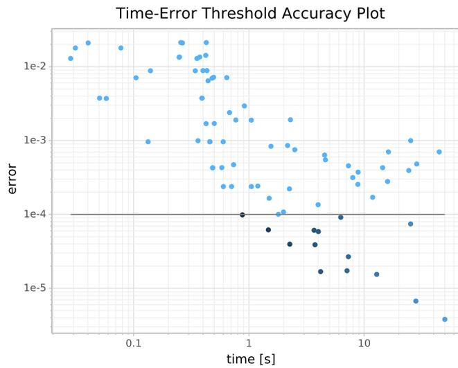
Figure 4.9.: Error threshold. All configurations above the line are considered invalid. Among the remaining, the ones with the lowest runtime are considered to have the highest quality.
