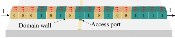
Fig. 1. RTM cell structure
