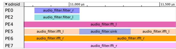
Figure 5: Visualization of the simulated execution of an audio filter application on the ODROID-XU4.
