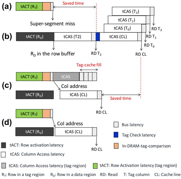
Fig. 10. (a) Super-segment miss detection in the tag region for the bypassed super-segment (b) Hit/miss latency in the baseline combined tag-data region (c) Hit latency of the decoupled design where tag and data regions are accessed concurrently along with tag-cache fill (d) In-DRAM tag comparison in [25] without a tag-cache.
