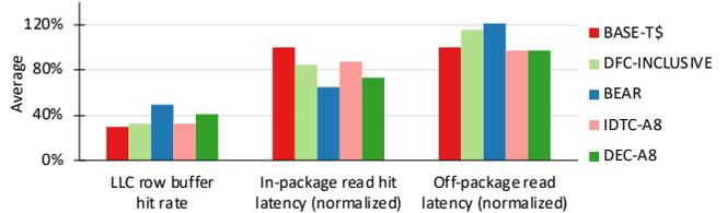
Fig. 15. LLC row buffer hit rate, hit latency and off-package read latency. All results are averaged across all workloads
