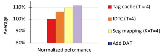
Fig. 18. Impact of individual contribution on performance. IDTC represents the decoupled tag-data configuration with selective in-DRAM-tag comparison for  $T=4$ .
