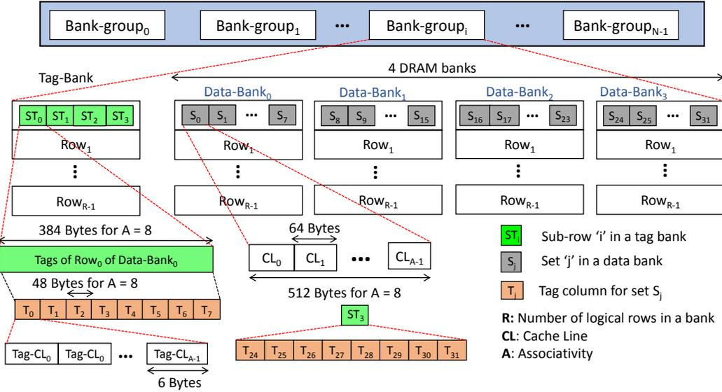
Fig. 5. Logical organization of the *decoupled cache* design
