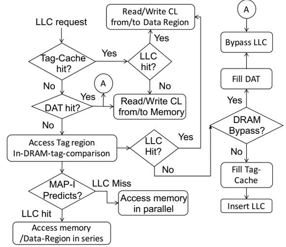
Fig. 9. DRAM LLC control flow with DAT and tag-cache
