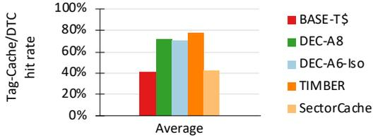
Fig. 14. Tag-cache/DAT hit rate results (DAT is not employed in BASE-T\$, TIMBER and SectorCache)
