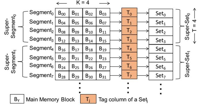
Fig. 7. Segment mapping to the tag columns.  $K$ : Segment size
