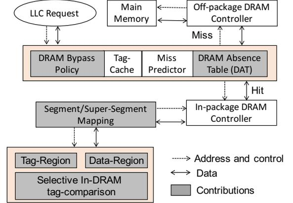
Fig. 4. High level view of our *Decoupled Cache Design*.
