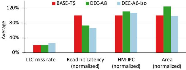
Fig. 19. Performance comparison of the iso-area *decoupled cache* (DEC-A6-ISO) with DEC-A8 and BASE-T\$
